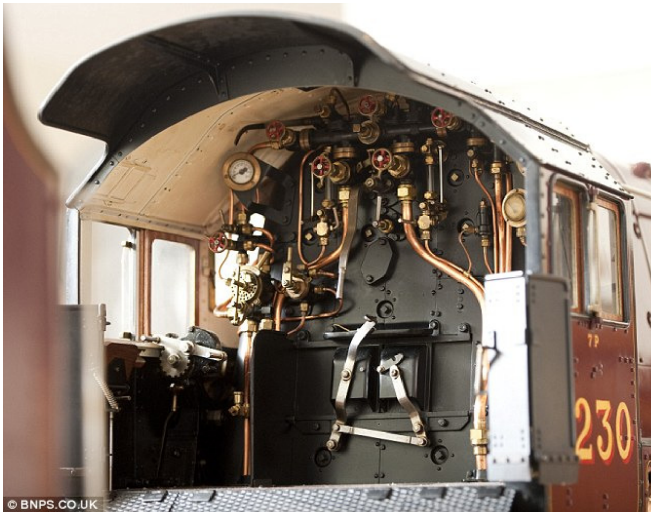
The Duchess was constructed by Harry Powell, who worked all his life at the Crew locomotive works and used his original drawings to make it. The fine attention to detail is such that it is fitted with a copper boiler, safety valves, regulator, blower, whistle, brake, wheel reverse gear, lever-operated sliding firedoors, pressure gauges, twin water sight gauges and a mahogany planked floor
