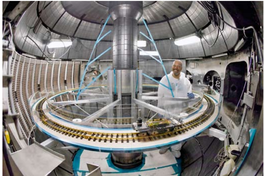
PPPL technician Sly Vinson installs the tracks inside NSTX. Photo credit: Elle Starkman
