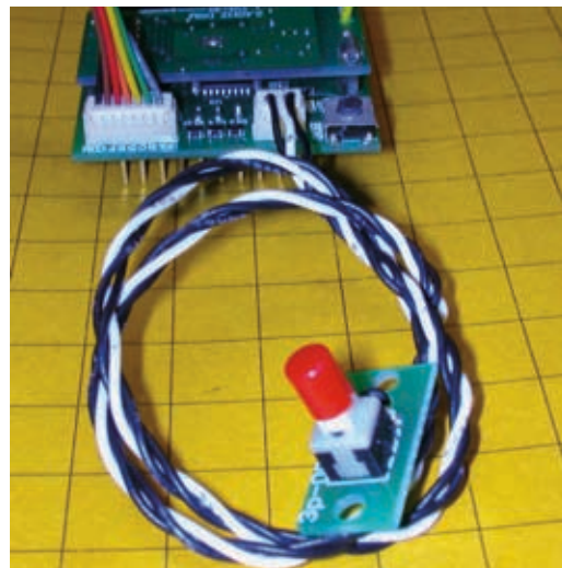
(fig. 7 - Close-up of the bind switch)
