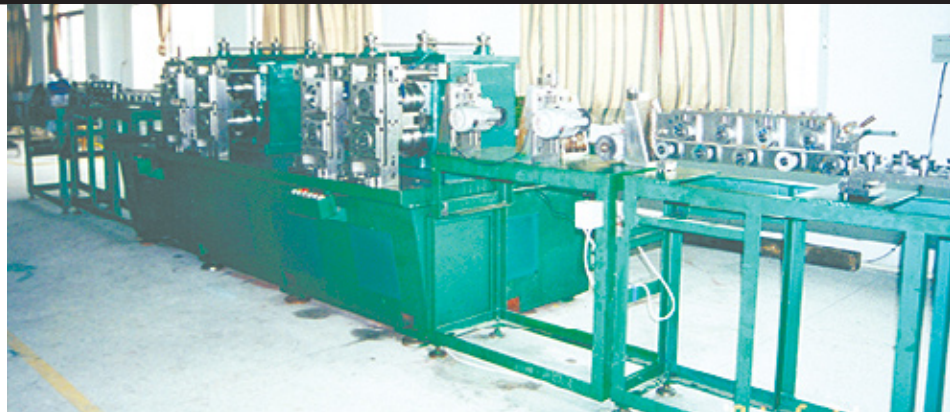
Aristo-Craft Stainless Steel Track Rolling machine
