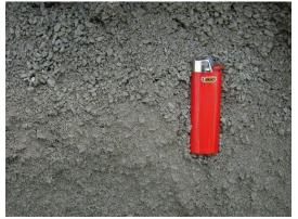
As you can see the 1/4" and under has a good bit of very small particles as well as the 1/4" size pieces. Once laid down, a good rain causes the fine particles to sort of bond together almost like mortar. I place my ballast in my trench and walk on in to compact it. I then wait for a good rain to cause the ballast to "settle". I then add more ballast to bring any low sections up to grade and then lay my track.
